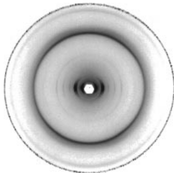
Figure 14. WAXD fiber pattern for CPEI(A) with anomalous orientation behavior. Fiber direction is vertical on the page.
